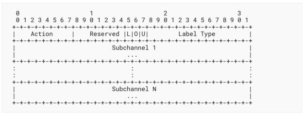
A LABEL-SET TLV represents a set of possible labels that can be used on an interface. If the L bit is cleared, the label allocated on the first endpoint **MUST** be within the label set range. The Action parameter in the LABEL-SET indicates the type of list provided. These parameters are described by [RFC3471], Section 3.5.1.
