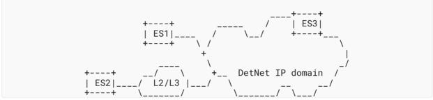
Figure 3: Connection Types of L3 End Systems
