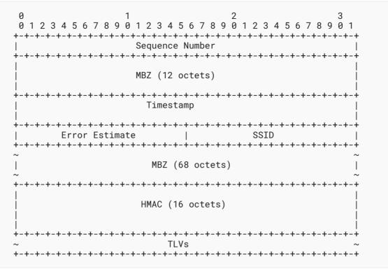
Figure 3: The Format of an Extended STAMP Session-Sender Test Packet in Authenticated Mode
