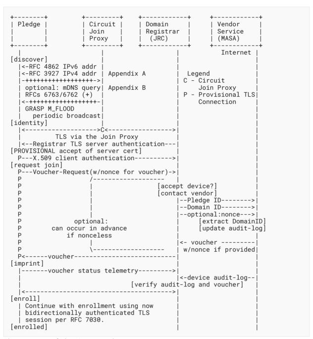
Figure 4: Protocol Time Sequence Diagram
