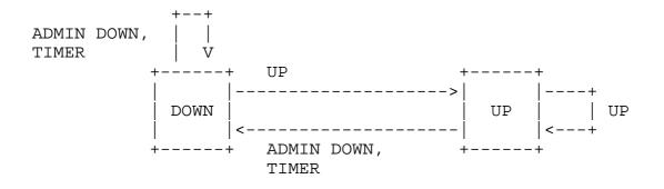
Note that the above state machine is different from the base BFD specification[RFC5880]. This is because the Init state is no longer applicable for the initiator of the S-BFD session. Another important difference is the transition of the state machine from the Down state to the Up state when a packet with State Up is received by the initiator. The definitions of the states and the events have the same meaning as in the base BFD specification [RFC5880].
