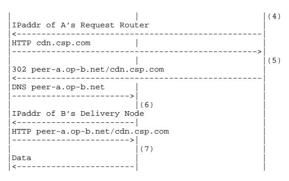
Figure 8: Message Flow for Content Pre-Positioning
