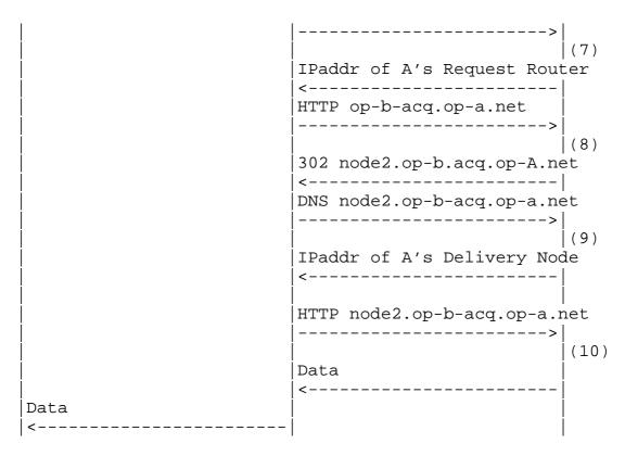
Figure 3: Message Flow for Iterative HTTP Redirection
