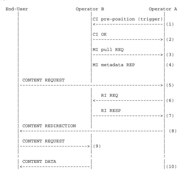
Figure 9: Message Flow for Asynchronous CDNI Metadata
