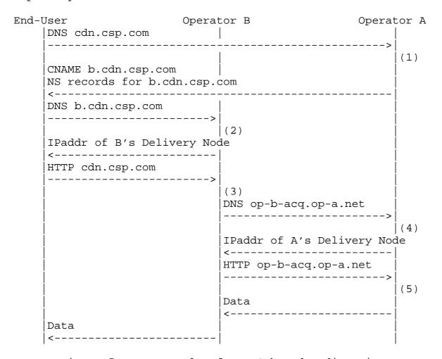
Figure 5: Message Flow for DNS-based Redirection
