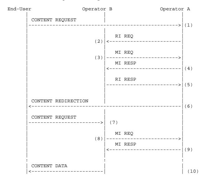
Figure 10: Message Flow for Synchronous CDNI Metadata Acquisition The steps illustrated in the figure are as follows:
