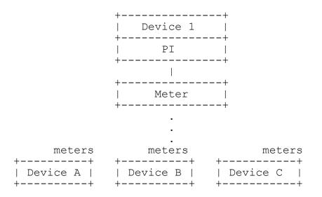
An analogy to communications networks would be modeling connections between servers (meters) and clients (devices) when the complete Layer 2 topology between the servers and clients is not known.
